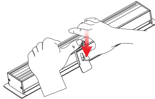
2 One hand to hold the spring buckle and the other hand to press it down harder (as shown in the figure)
