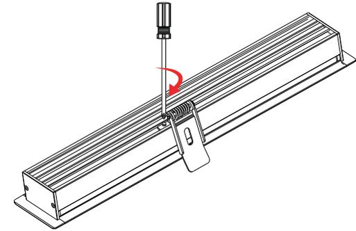
3 Tighten the screws. Installing other buckles in the same way
