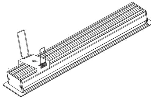
2 Moving the buckle to another side of slot and stuck into it
